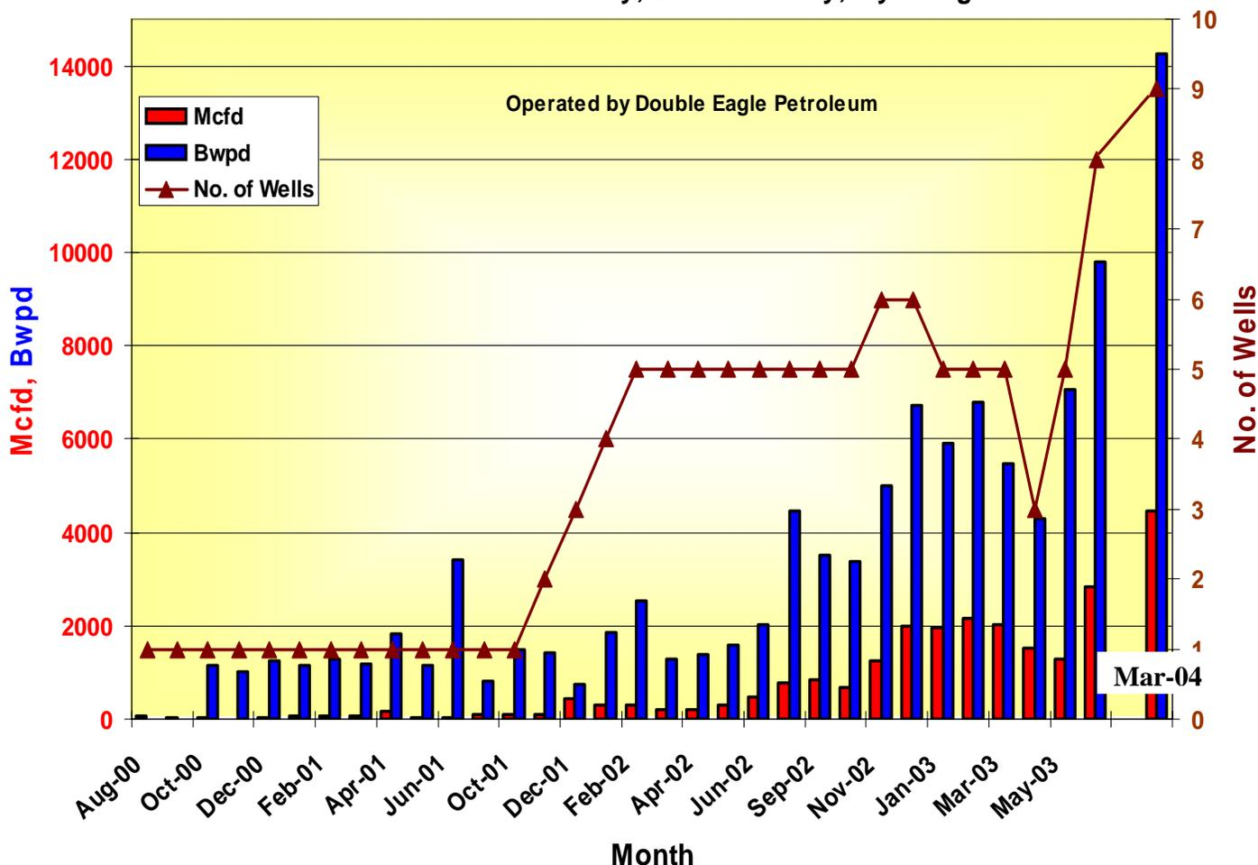
**Figure 1.** Nine wells produced 4453 Mcfd and 14,240 Bwpd at Cow Creek Field during November 2003.
