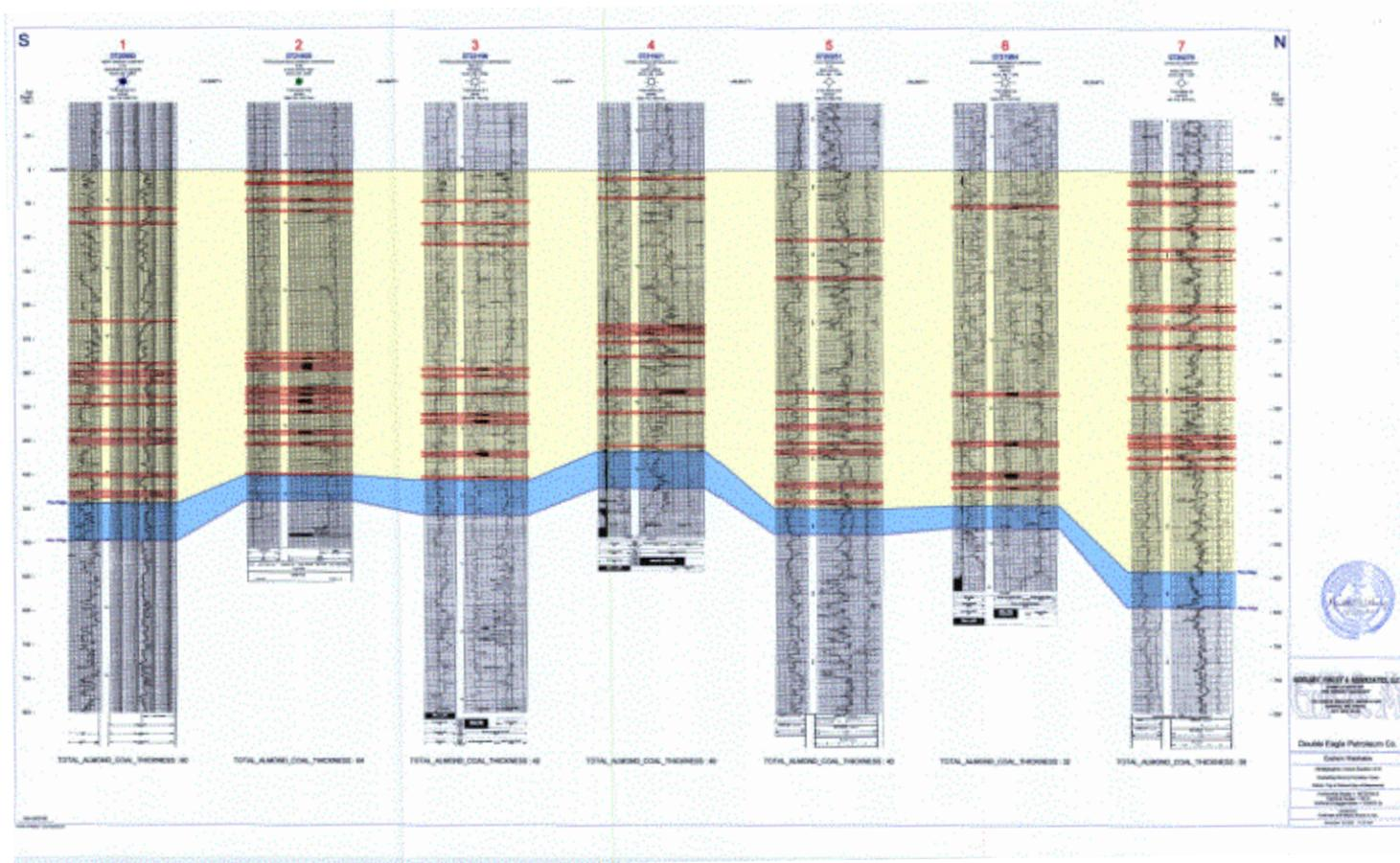
**Figure 3.** Log cross-section showing continuity of Almond coals across Cow Creek Field. Coals are highlighted in red and marine shoreline sandstone is shown in blue.
