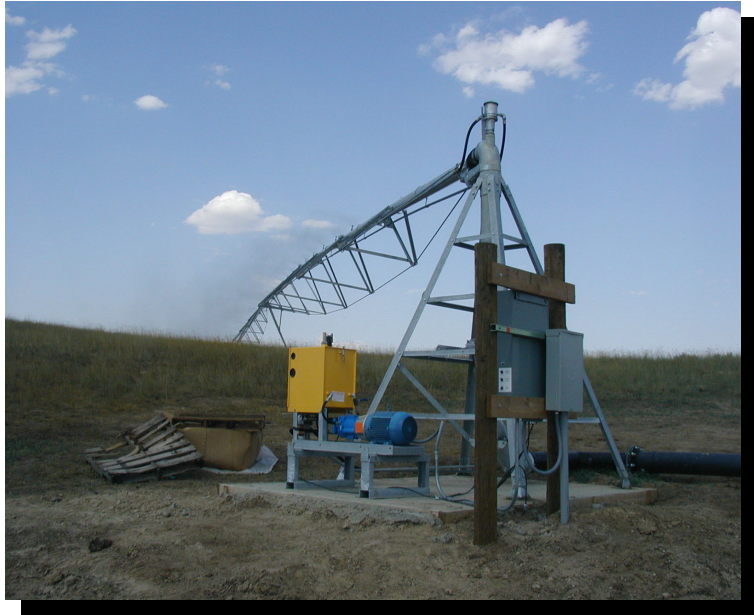
A center pivot irrigation system is a self-propelled irrigation system that rotates around a central, fixed pivot point.
