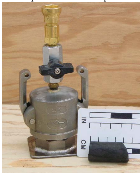
Figure 10. Rotary sidewall coal core and sidewall canister.
