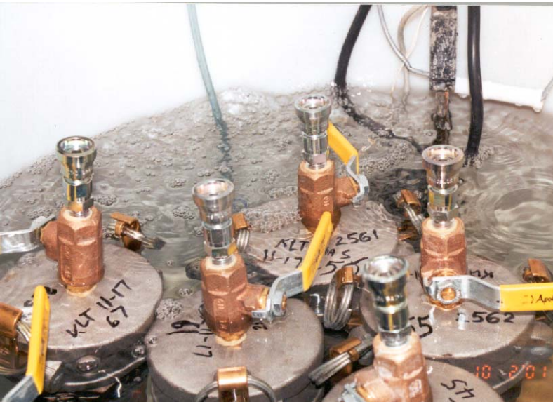
Figure 4. Water bath for maintaining canisters at a constant reservoir temperature.
