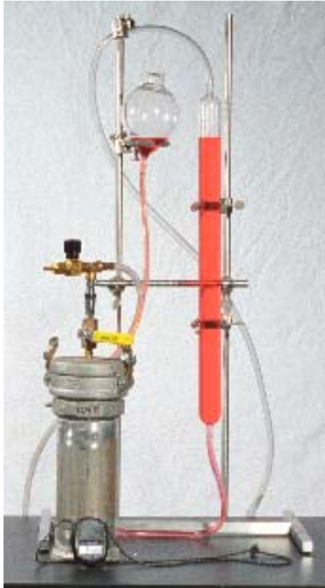
Figure 3. Desorption canister, barometer, and burette for taking gas readings. Size of burettes vary depending upon expected gas amounts.
