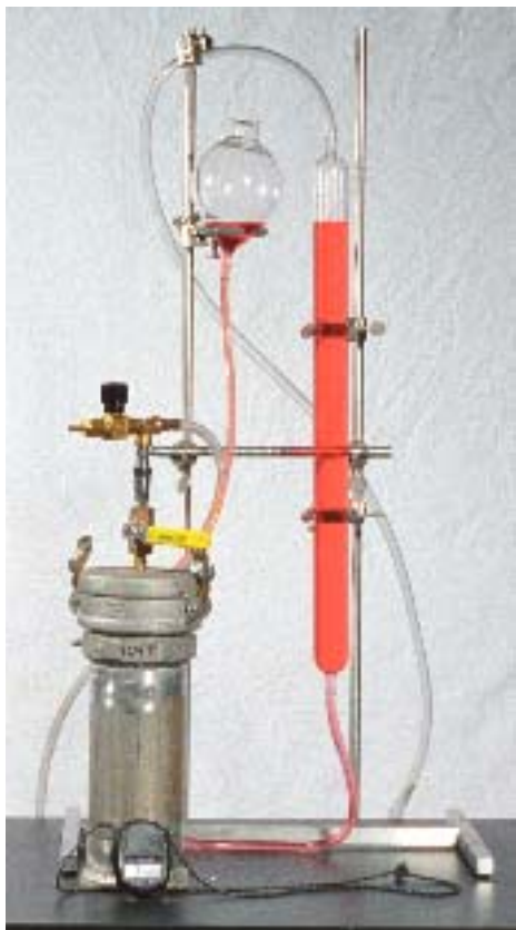
Figure 1. Typical desorption setup: air-tight canister with valves, burette, and barometer.
